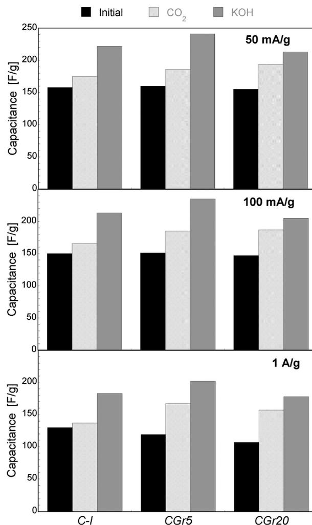
Figure 6. Comparison of the capacitance at different current loads in  $\text{H}_2\text{SO}_4$  as an electrolyte for the initial samples<sup>32</sup> and those activated with  $\text{CO}_2$  and KOH.
