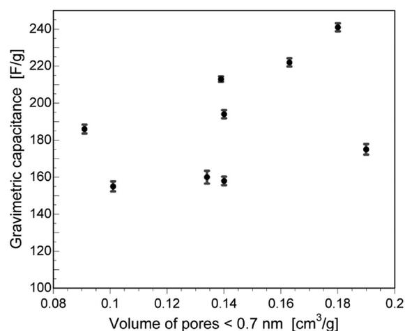
**Figure 8.** Dependence of the capacitance in  $\text{H}_2\text{SO}_4$  on the volume of pores smaller than 0.7 nm.
