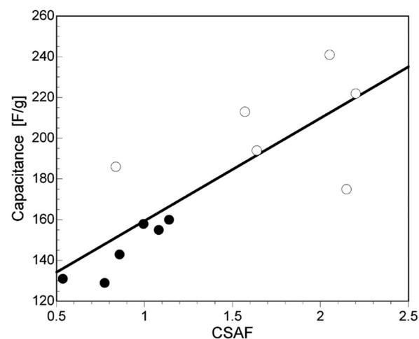
**Figure 9.** Dependence of the capacitance measured in  $\text{H}_2\text{SO}_4$  on the CSAF. The data from ref 32 is marked as dark symbols.
