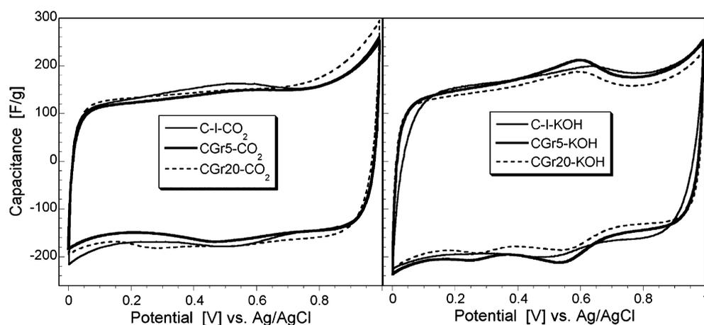
**Figure 4.** CV curves in three electrode cell vs Ag/AgCl at scan rate 5 mV/s in H<sub>2</sub>SO<sub>4</sub> as an electrolyte.
