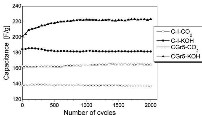
**Figure 10.** Specific discharge capacitance during galvanostatic cycling at 1 A/g in 1 M H<sub>2</sub>SO<sub>4</sub>.
