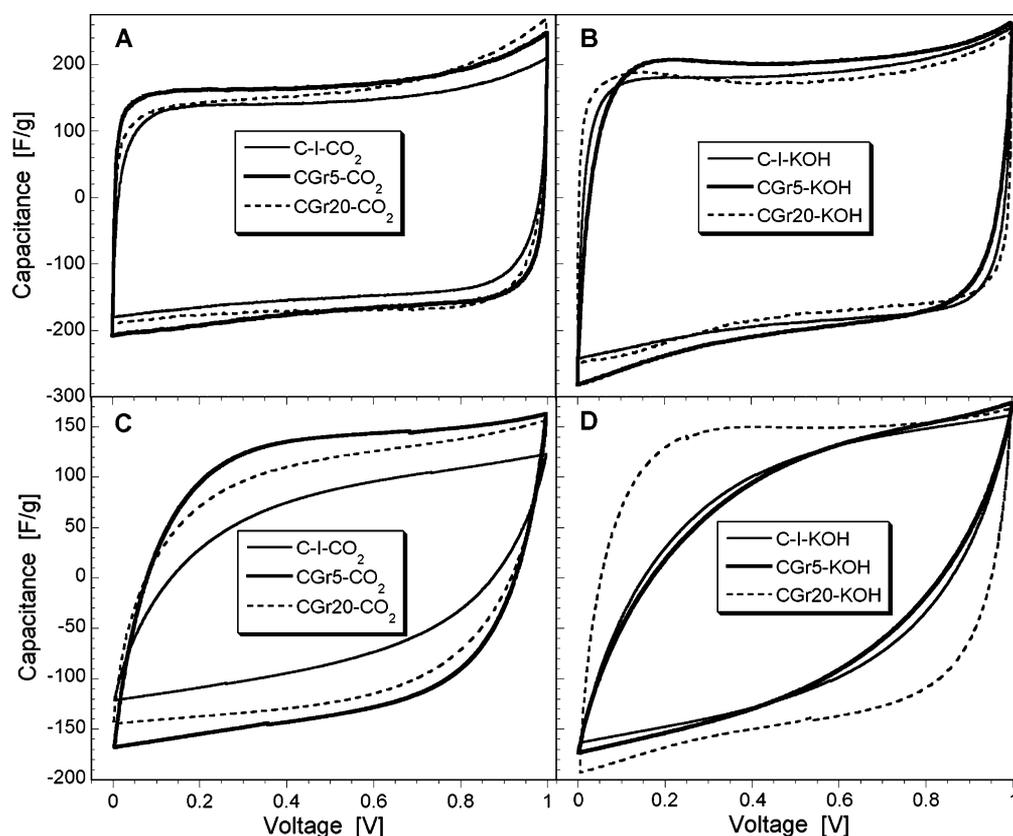
**Figure 3.** CV curves in two electrode cell at different scan rates in 1 M H<sub>2</sub>SO<sub>4</sub> as an electrolyte: 5 mV/s (A, B) and 100 mV/s (C, D).
