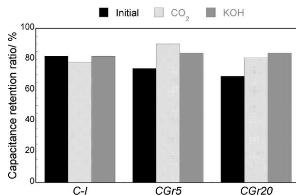
Figure 7. Comparison of the capacitance retention ratio in  $\text{H}_2\text{SO}_4$  for the initial samples<sup>32</sup> and those activated with  $\text{CO}_2$  and KOH.
