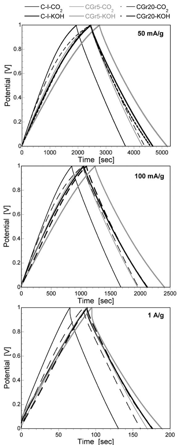
Figure 5. Charge/discharge profiles at different current loads in  $\text{H}_2\text{SO}_4$ .
